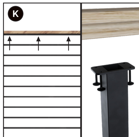
Drill 1/8" pilot holes Use 1-1/4" handrail screws
